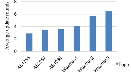
Fig. 4. Average update round grows with network size when the percent of saved-energy is fixed for energy-saving driven updates.
